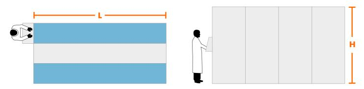
LENGTH from 3 meters to 15 meters - HEIGHT from 2 meters to 4 meters - WIDTH 1,43 meters: thanks to the modular nature of Sintesi, the robot can be adapted to any pharmacy space. Customized solutions can be designed upon request. Sintesi is the most compact robot in its category.
